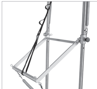
Figure 6: Safety strap holding the push-through bar at 4 o'clock. The strap is secured to the PTB and canopy frame, not the eyebolts.
